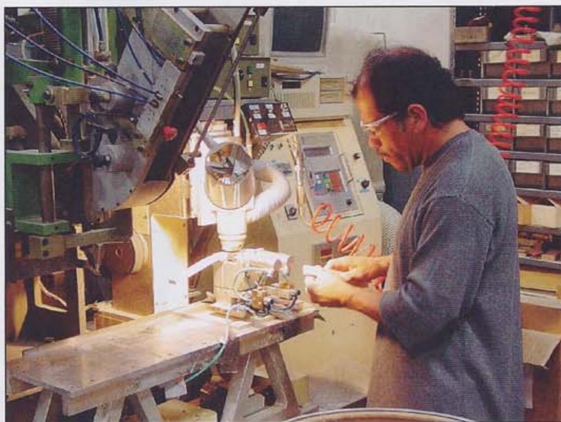
Francisco Martinez is shown operating a brush making machine which is drilling holes into brush handles.
