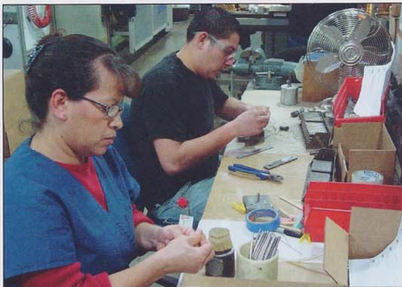
Guadalupe Limas is shown filling a stainless steel tube with horsehair material, while William Diaz is filling a steel tube with carbon steel material. Both materials are used for applicator brushes.
