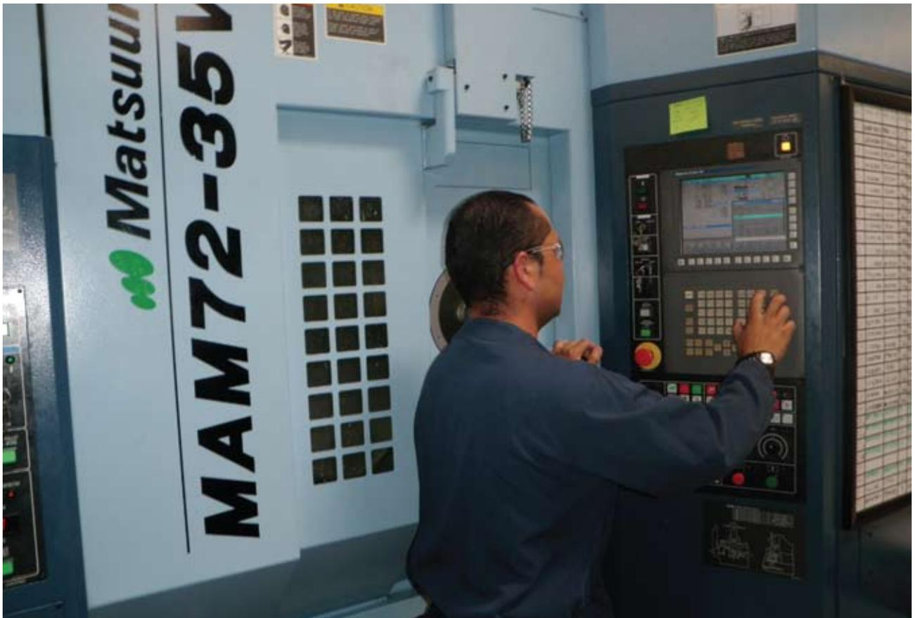
**An engineer at True Position Technologies sets up an operation on a Matsuura VMC.**
