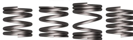
(C) Closed & Square (CG) Closed & Ground (DC) Double Close (O) Open
