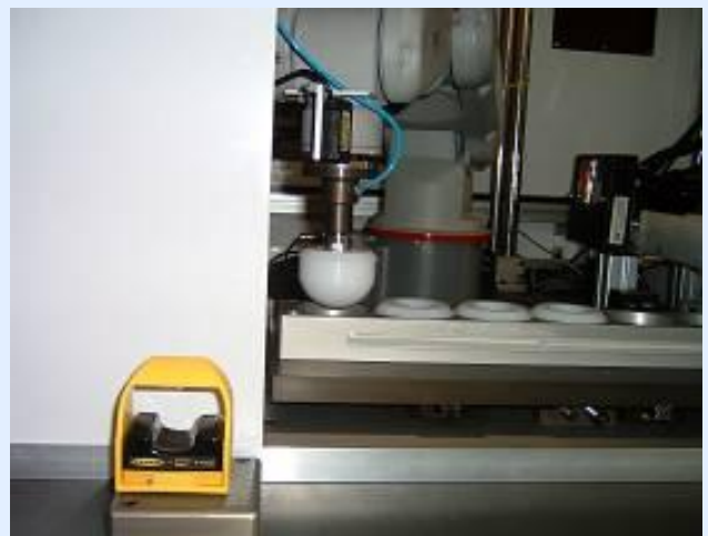
6-Axes Robot with part present sensor for automatic pick & place
