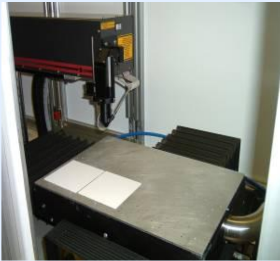
Fixed Beam Delivery System with Programmable X-Y-Z axes for Cutting & Scribing applications
