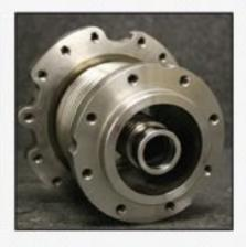
BMR expansion joints are used in a wide variety of piping applications to compensate for thermal pipe expansion or contraction, and to absorb equipment vibration or pipe motions. These products provide piping system flexibility under extreme operating conditions. BMR manufactures single, multiply, and two-ply testable bellows in sizes from 0.5" to 36" in diameter using precision forming technology.
